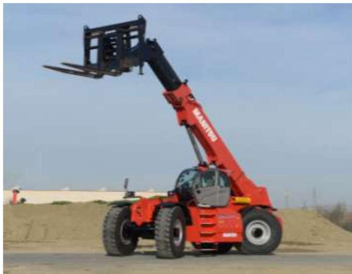
There is also a substantial range of mining attachments, with a fork positioner (width 2,900 mm) with side shift and a capacity of 33 t to 12 m. Designed specially for the high tonnage MHT 12330 telehandler, this positioner assists in the handling of heavy loads used in mines (including spare parts).
